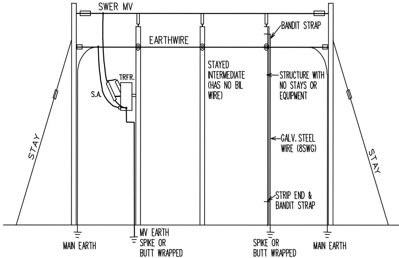
SWER LINES WITH EARTHWIRES FOR INSIDE VILLAGES AND TRANSFORMERS CONNECTED
