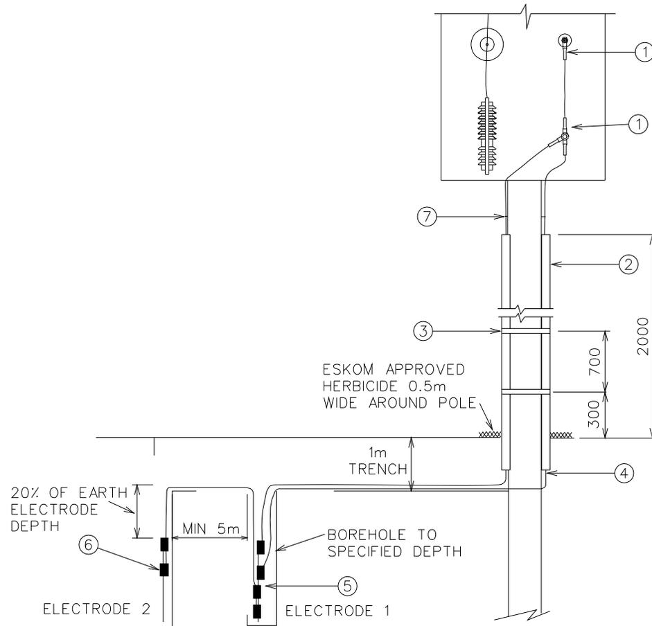
Transformer rod electrode installation
