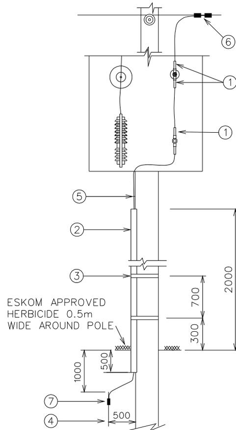
Transformer local redundancy earth.
