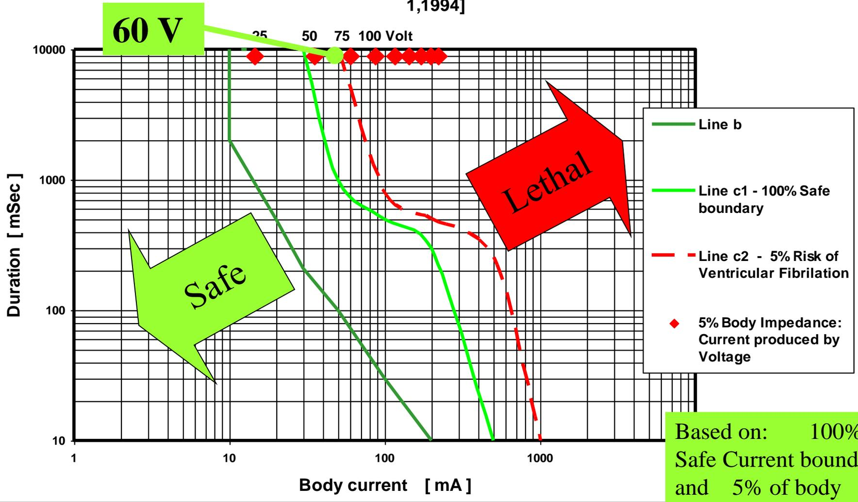
Based on: 100% Safe Current boundary and 5% of body resistance
